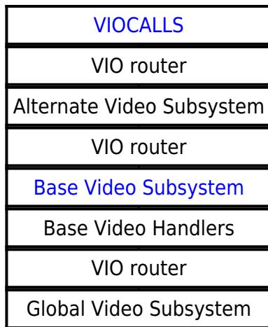
In late OS/2 versions (3.x?) actual code of Video subsystem and Base Video Subsystem was moved to DOSCALLS.DLL (see Fig). OS/2 Video Subsystem is 16-bit. Later three independent versions of 32-to-16 bit wrapper subsystems were developed (See Fig)
